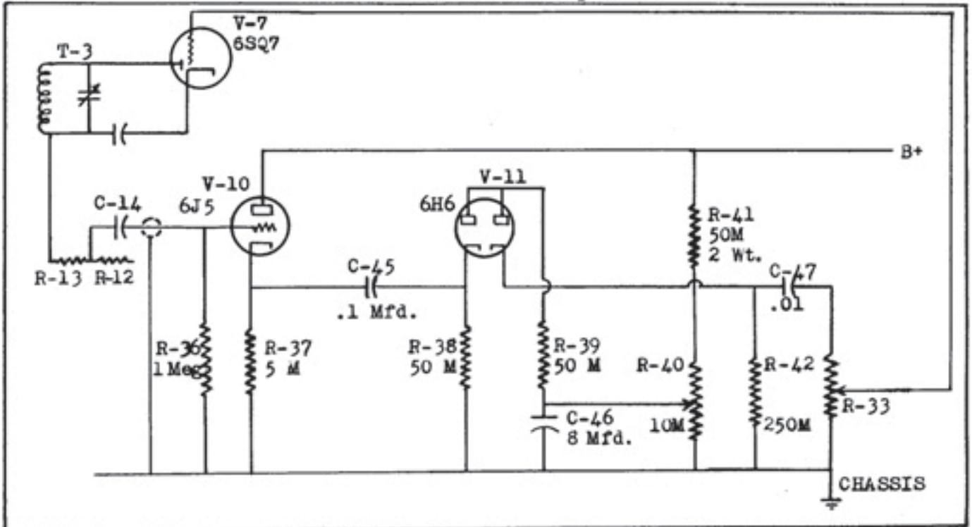
Schematic diagram illustrating Noise Limiter section of
